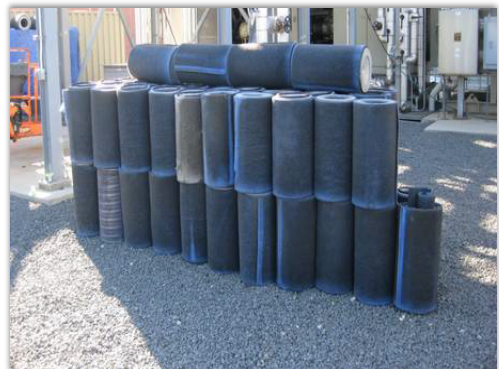
Competitive E10 filters spiked in pressure after six months of service
