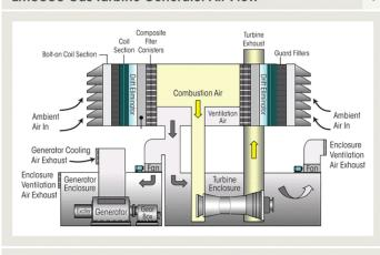
use a three-section inlet air filter that mounts directly above the turbine enclosure, conserving space and providing compact, low-pressure loss ducting to the turbine inlet. Figure 1 provides an illustrative example.
