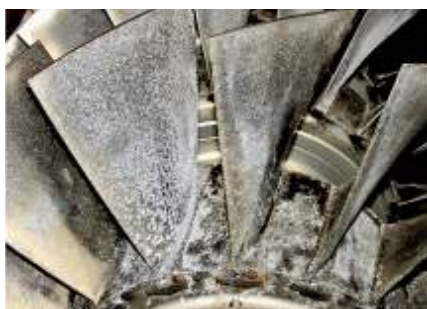
15MW Gas Turbine Forties Field with hot end corrosion failure circa 8,000 operating hours (2007), first stage compressor blades showing high levels of salt loading and blade damage.
