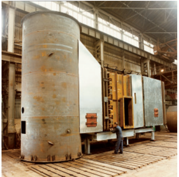
AAF built 21 exhaust systems for GE Frame 5 machines to be used on the Russian gas pipeline.
