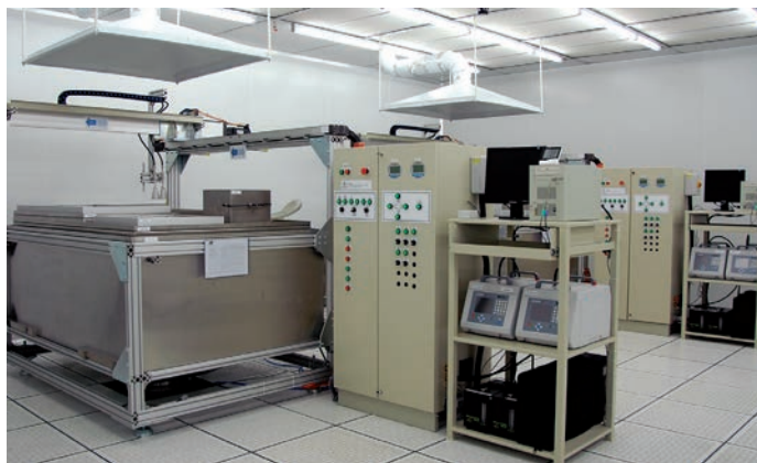
AAF laser spectrometer.
