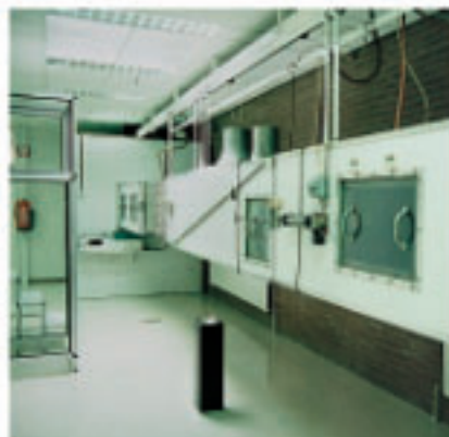
Performance testing in the EN 779 test dock.
