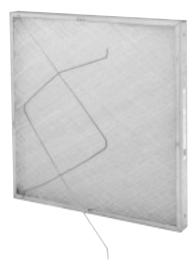
The cell sides are made from a single piece of 22-gauge, galvanized steel U-channel. They are available in 1"and 2" thicknesses sized to fit inside 2" deep universal holding frames, or in 1" and 2" side access housing tracks.
