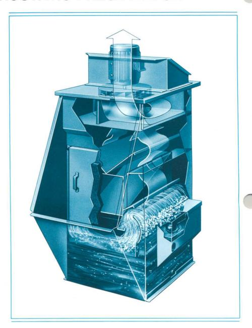
centrifugal force exerted by the rapid changes in direction of air flow causes the dust particles to penetrate the water droplets and become permanently trapped within them.
