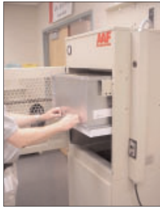
Filter should only be pulled partially out, to gain easier access to prefilter clips
