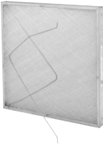
The cell sides are made from a single piece of 22-gauge, galvanized steel U-channel. They are available in 1" and 2" thicknesses sized to fit inside 2" deep universal holding frames, or in 1" and 2" side access housing tracks.
