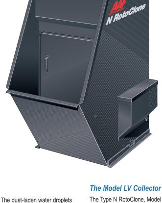
are then removed from the air stream by the water eliminator. The dust settles in the bottom of the collector and the water is reused. Since the water curtain is produced by the airflow, no pumps or nozzles are required.
