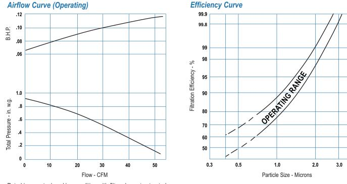
Rated in an actual working condition with filter element saturated with oil.
