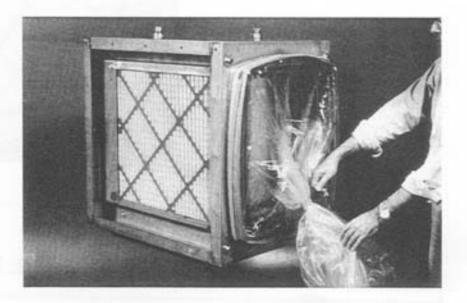
The bag includes a number of gloves which form an integral part of the bag. These are provided to facilitate manipulation of an internal filter clamping mechanism and handling of the filters. Locate the gloves.
