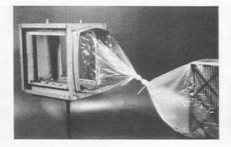
Using shears, cut the bag between the hose clamps. An alternate method is to use tape instead of hose clamps. The bag would be taped in three (3) places simulating the ties and clamps. Care should be taken to ensure that the bag is very tightly taped. The center tape is then cut to separate the portion of the bag with the filters from the portion attached to the enclosure bag mounting collar (this portion is known as the bag stub).
