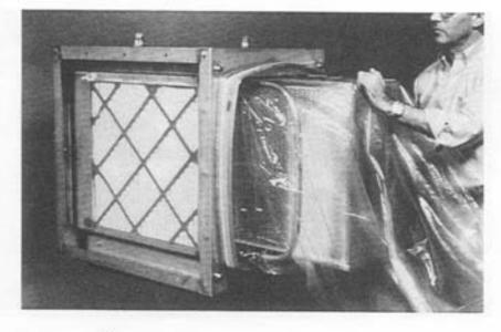
Clamp the HEPA filter into position. This will be the reverse of the operation described in Steps 6 and 7.
