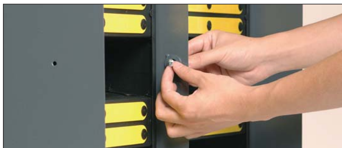
Step 2: Locate the channel against the left side of the center vertical cassette support panel, inside the locking handle support tab, with the channel legs facing away from the cassette.
