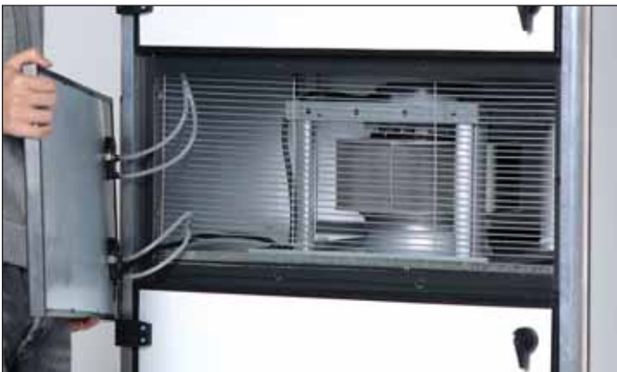
Step 4: Remove the safety grille to access the fan and motor.
