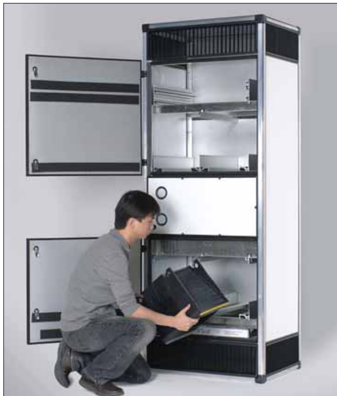
Step 1: Bring the HD half-cassette to the RU and prepare to install it. Turn the half-cassette so that the yellow butterfly gasket will be on the bottom and pointing into the enclosure.
