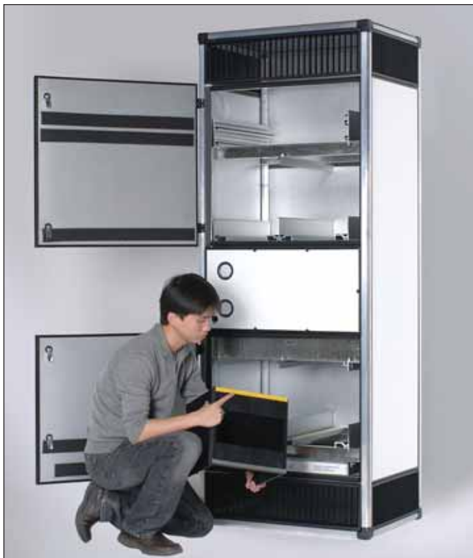
Step 1: Bring the HD half-cassette to the RU and prepare to install it. Turn the half-cassette so that the yellow butterfly gasket will be on the bottom and pointing into the enclosure.
