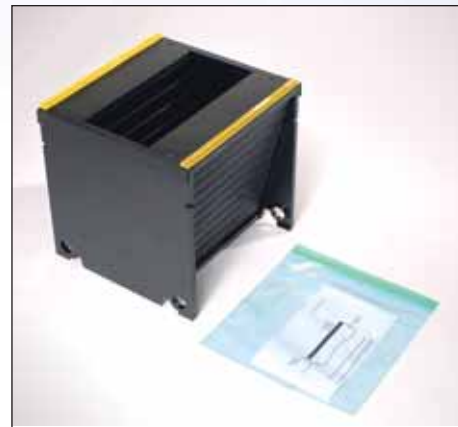
Step 4: The Type HD half cassette is now ready for installation into the RU.
