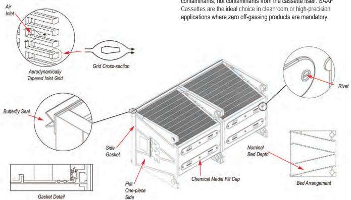
**SAAF-T-Butterfly Seal** and **SAAF-T-Groove** - Designs provide near absolute sealing, even in existing retrofit applications.
