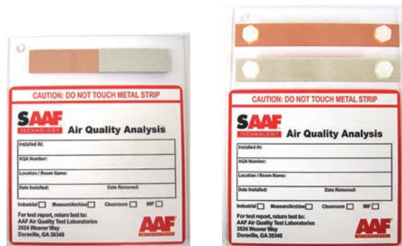
Metal Coated Glass Coupons
