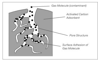
Figure 1 - Adsorption taking place on activated carbon
