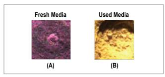
Figure 2 - Cross sections of permanganate media; (A) fresh permanganate media before reacting with contaminants: (B) used permanganate media after forming chemical bonds with contaminants.
